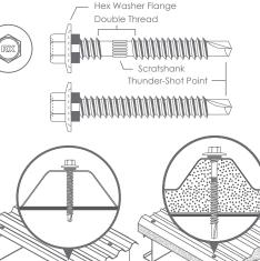
**DOUBLE THREAD** RX-SDHCG1245C3N 12-14 x 45mm RX-SDHCG1255C3N 12-14 x 55mm RX-SDHCG1265C3N 12-14 x 65mm
